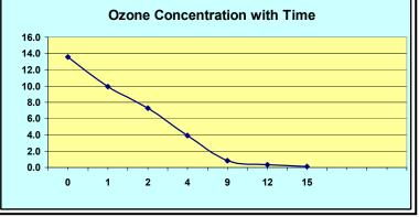
from 25 ppm down to 14 ppm, while the relative humidity went from 66% down to 52%. Following the soak period the catalytic scrubber was turned on and the ozone concentration was reduced from 14 ppm down to 0.2 ppm.
