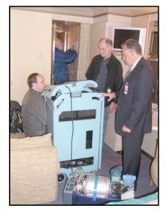
The ViroForce ozone generator/catalytic-scrubber prototype and the rapid humidifier prototype were placed on the floor within the cabin as shown in the photo to the left. Room vents were sealed off with duct tape to prevent any ozone from escaping the cabin. The cabin dimensions were measured and the cabin volume was calculated to be 1308 cubic feet.
